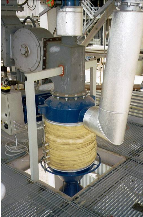
32. picture – Fly ash dry unloading - Steyrermühl, Austria
