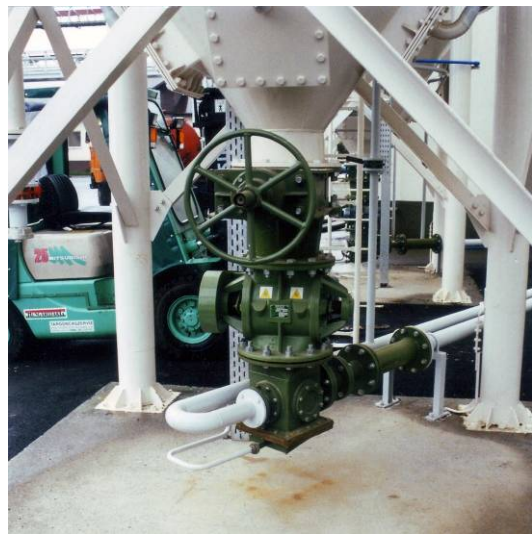
19. picture – Perlit conveying with pneumatic jet pump – Martfű, Hungary
