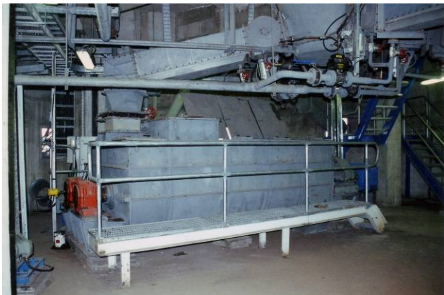
33. picture – 200 TPH double screw paddle mixer - Suralaya, Indonesia
