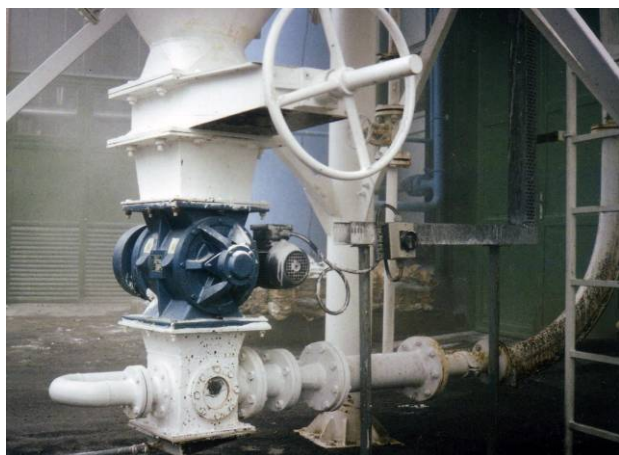
20. picture - Perlit conveying with pneumatic jet pump – Martfű, Hungary
